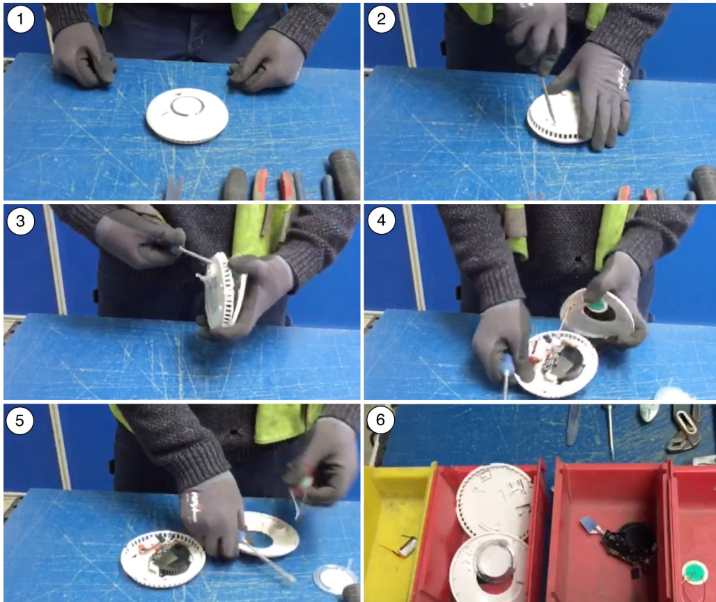
Figure 7: Manual disassembly of a fire alarm
