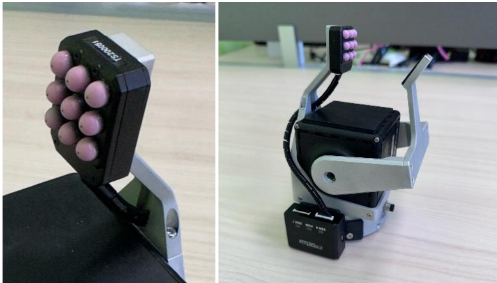
Figure 7 Mechanical integration of tactile sensor array on VS Gripper
