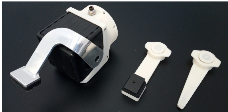
Figure 8: VSA gripper with the tool exchange system and different tools
